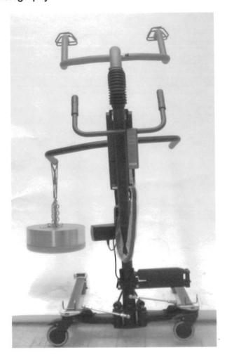
A considerable deformation took place and the hoist was close to tipping sideways as long as the load was applied. From the photography may be seen that the right rear wheel ha been lifted approximately an inch from the floor.
